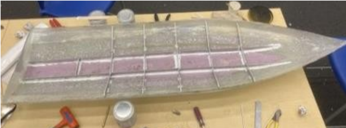
Figure 4: Bottom section of the hull showing alignment of aluminum stringers
