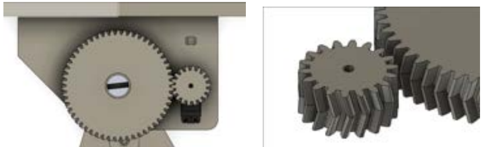
Fig. 3: The left shows the positioning of the geartrain, the right shows the herringbone gear type that was chosen.
