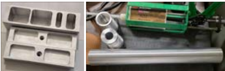
Fig. 11: Select manually machined steering and midsection components.
