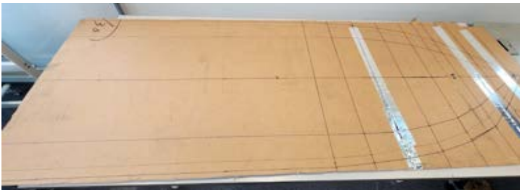
Figure 3: Frame sketches transferred from CAD model
