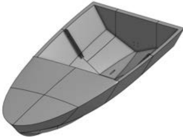
Figure 1 – Deep-V hull CAD model showing the interior geometry and printed section layout
