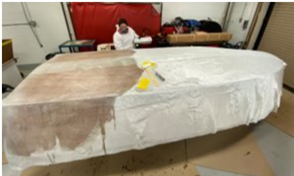
Figure 3: Fiberglass Laying on Outside of Vessel
