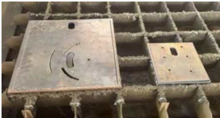
Figure 10. CNC Plasma Cut Plates for Gearbox
